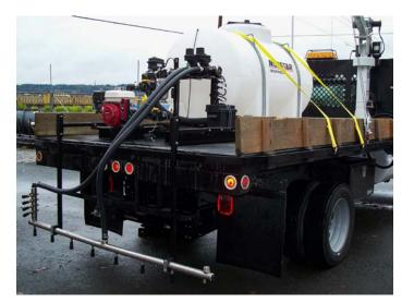
Standard skid mounted units are available with 300, 500, 750 and 1000 (larger tanks available upon request) gallon capacity poly tanks which include a Surge Buster baffle system. The skid and tank-saddle is constructed as an integral unit with formed longitudinals. All skids are powder coated and include forklift receivers and 4 lifting eyes (tie-downs). Optional telescopic storage leg stands and hooklift subframes are available.
