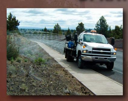
The sprayhead uses solid stream nozzles and a nutating motion to provide blanket coverage out to 28 feet wide. An optional 8th section can be added to increase the coverage to 36 feet.
