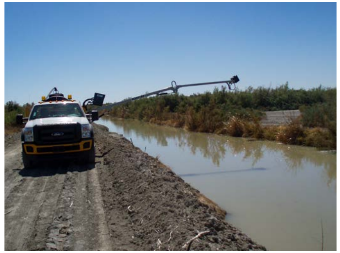
Articulated booms with boomless nutating sprayheads will substantially increase spray width capability.
