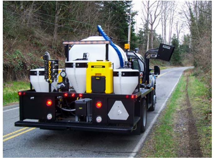
Standard chemical injection sprayers available skid or chassis mounted.
